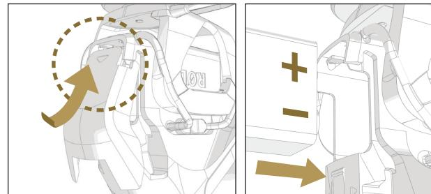
Installing the battery
